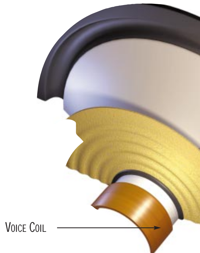
Figure 1. The construction of a cone assembly, showing the diaphragm connected to the voice coil that drives it, and spider and surround that support it.
