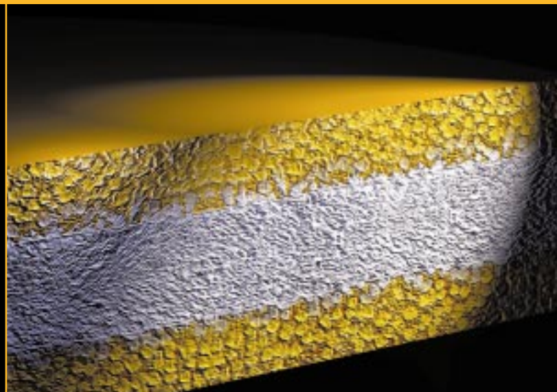
Figure 4b. An electron microscope photograph showing a cross section of a C.M.M.D. cone.
